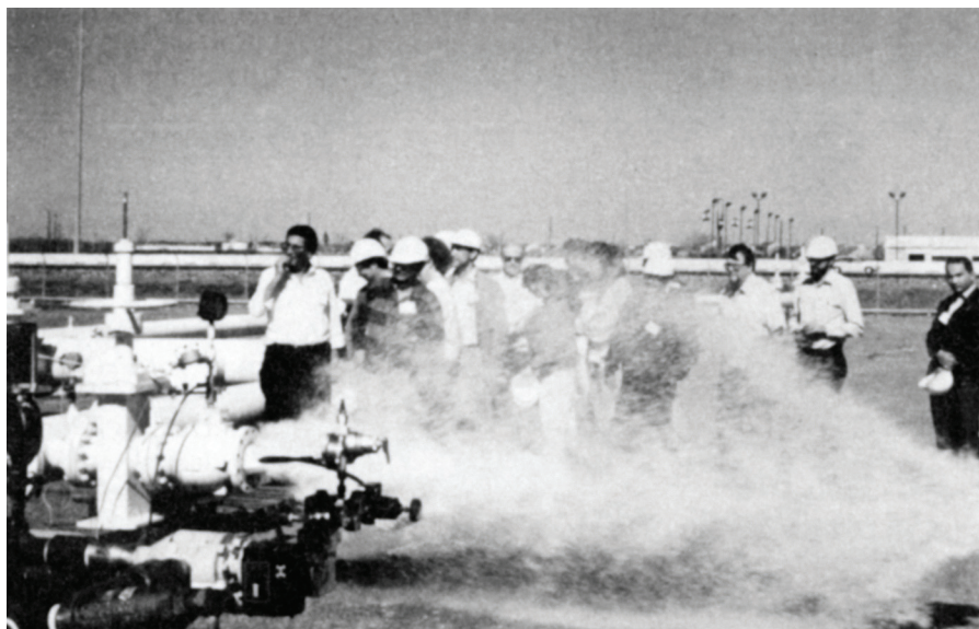
Fig. 7. Axial flow surge relief valve in test loop.
